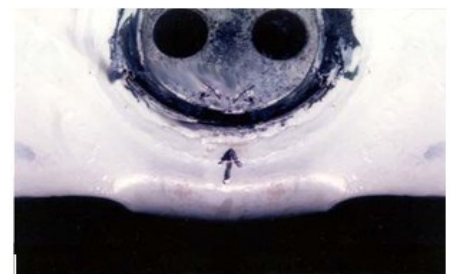
Photo 2: Close-up of worn bushing.
