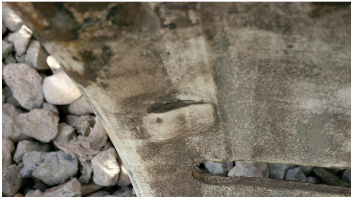
Even though light can be seen between the raised portion of the stop and the rim base, this is not damage
