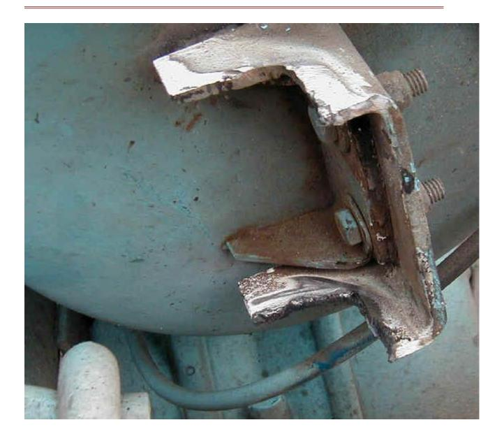
Trim back connecting welds at the front/outside/rear of spring hanger and under the slider retainer
