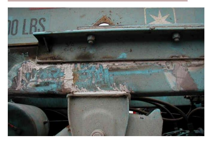
Scarf air tank bracket loose from frame
