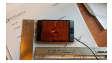
Please note that the Peterson 215 looks like a 2 ½ inch rectangular reflector (available in either red or amber) and contains a single LED light in a self-grounding enclosure. It has a height of less than 1.0 inch. Since this light also contains a reflector it will also eliminate the need for an adjacent reflector.
