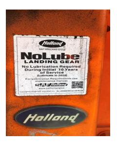
It has come to our attention that despite being clearly labeled that these legs do not require additional lubrication for several years, they are being routinely lubricated as part of FMCSA servicing.
